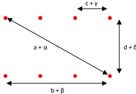
Within the recommended wavelength range, the zeroth order has a significant lower power than the desired diffraction orders of the dot matrix. Pattern size and pattern angles, and the ratio between central spot / zeroth order and desired orders will vary most with the wavelength. Diffraction efficiencies given on this datasheet have been measured using elements of product revision A.
