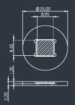
25 mm anodized aluminum mount with 8.95 x 8.55 mm clear aperture
